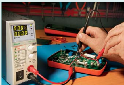
Current limited DC supply for electronic repair and calibration
