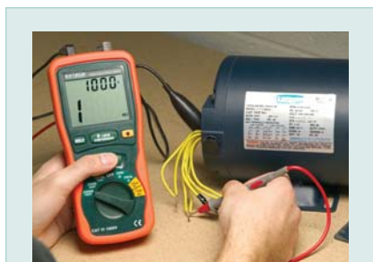
Measures the insulation resistance of motors
