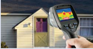
Infrared cameras quickly locate moisture related problems
